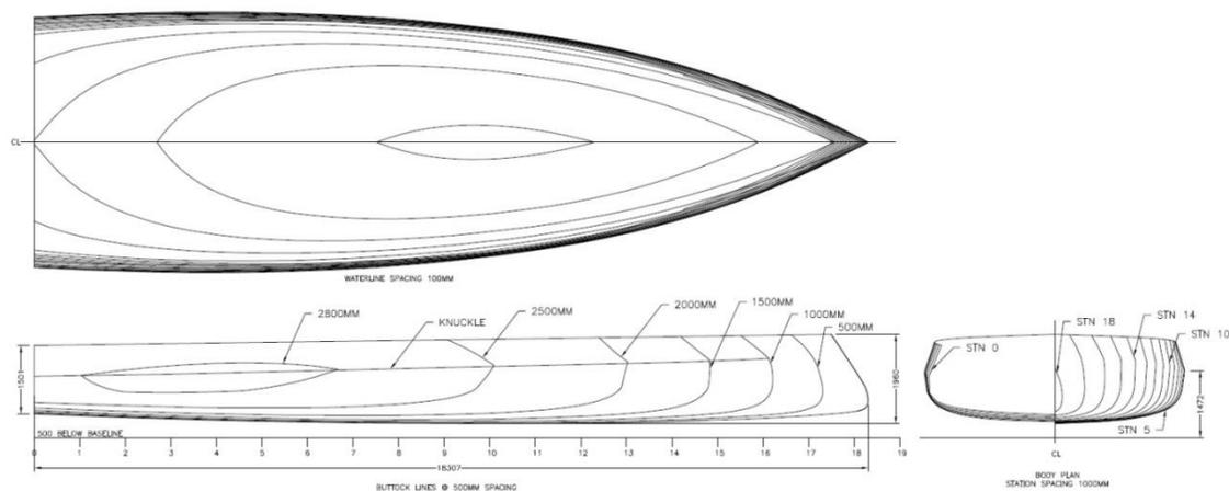
Figure 4: The Type 600 Lines Plan
