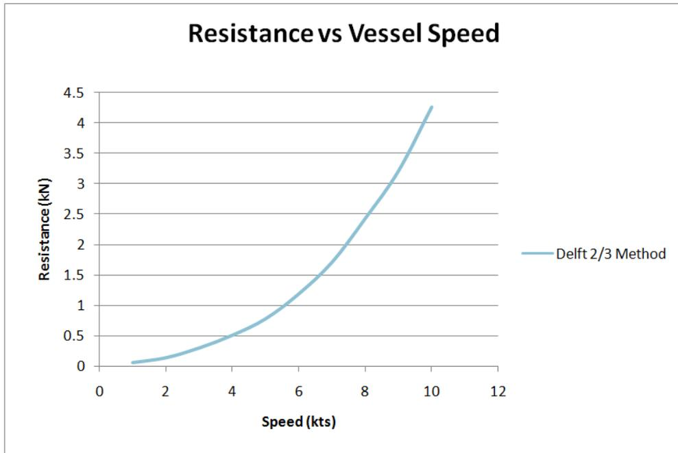
Figure 65: Resistance vs Ship Speed
