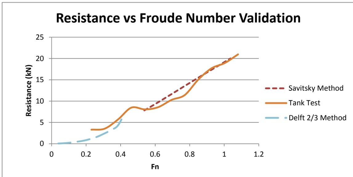
Figure 25: Compare Tow Tank Resistance with NavCAD Methods (NavCad, 2014)
