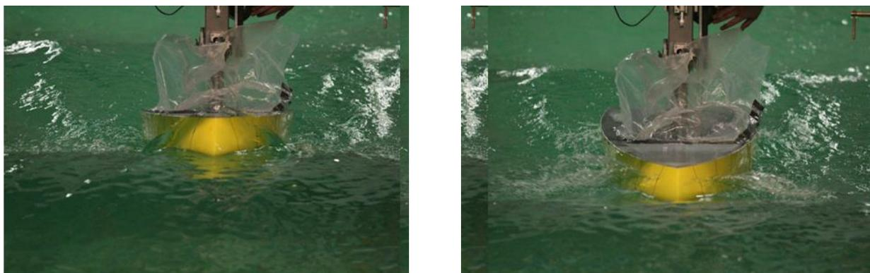
Figure 23: Unballasted condition at 18 knots with 0 degree heel and 0.6 Hz wave. (Photo Credit to Ryan Williamson)
