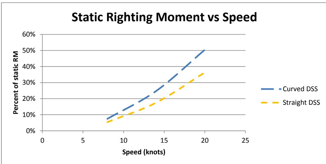
Figure 53: Righting Moment vs. Speed (10 degree Heel)
