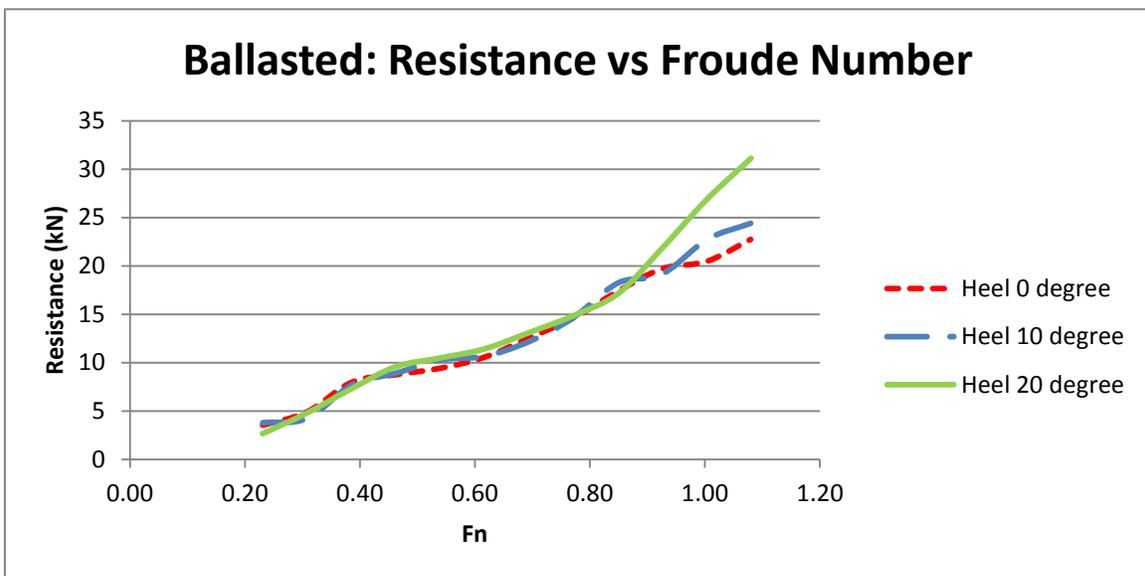
Figure 20: Resistance vs Froude Number in Ballasted condition
