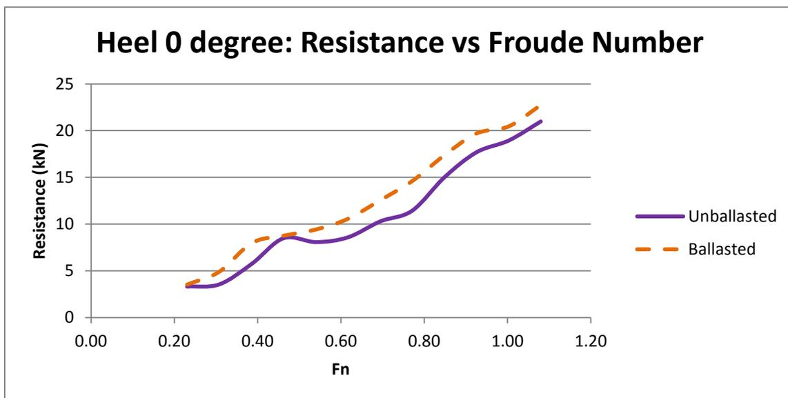
Figure 16: Resistance vs Froude Number at 0 degrees heel
