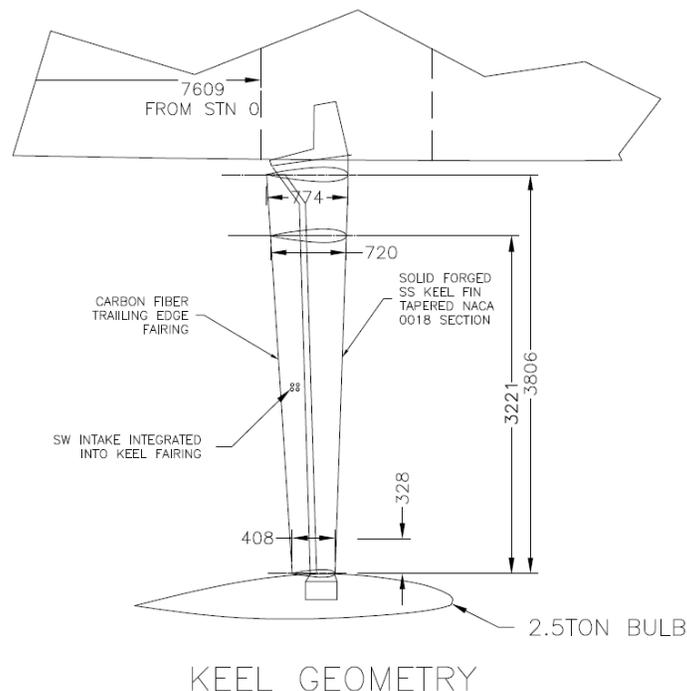
Figure 58: Keel Fin geometry with SW intake
