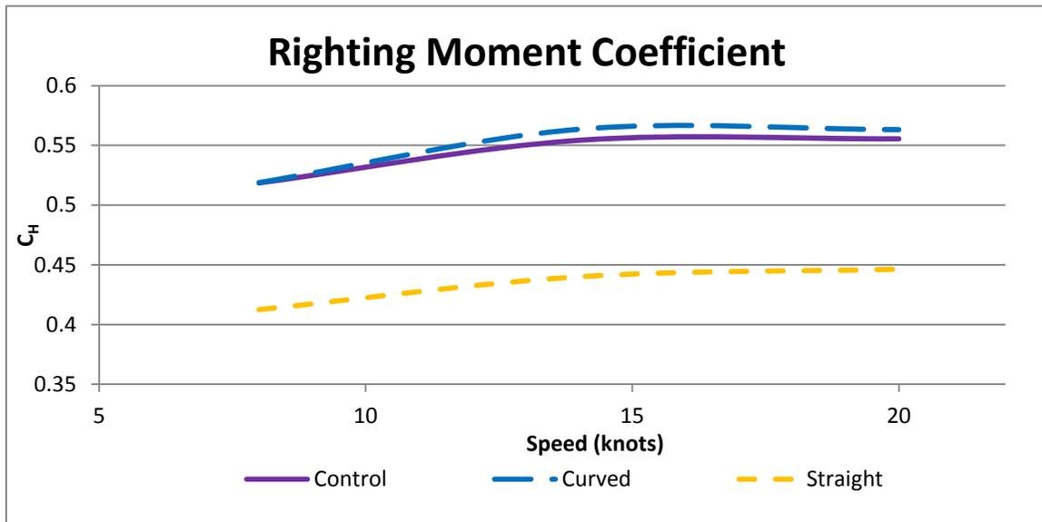
Figure 51: Righting Moment Coefficient vs Vessel Speed
