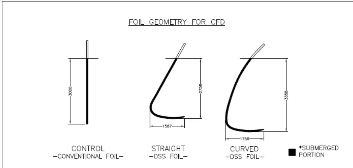
Figure 46: Three Foil Types Analyzed in CFX
