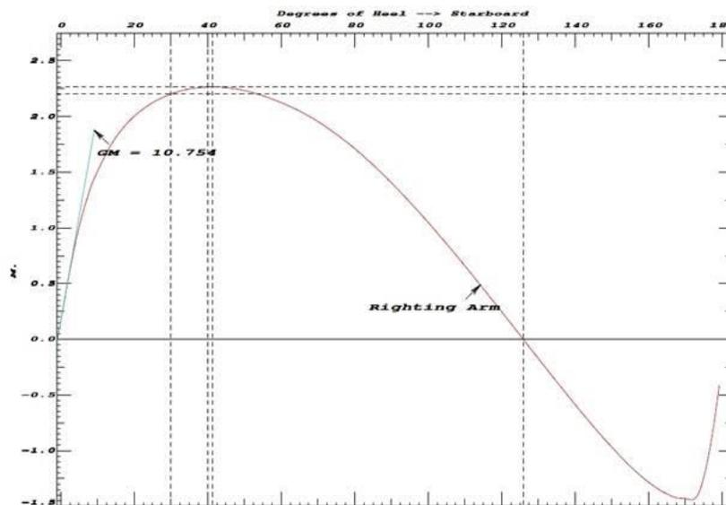
Figure 9: Righting Arm curve for 5 degrees cant
