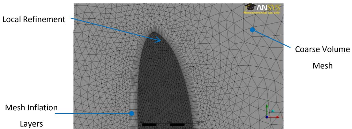
Figure 47: Local refinement and inflation layers
