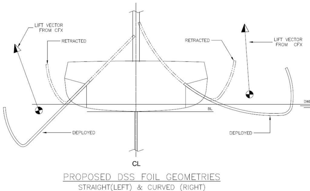
Figure 44: Proposed DSS Foil Geometries
