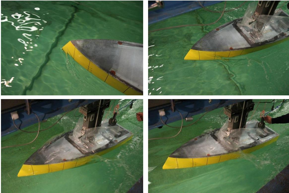
Figure 22: Ballasted condition with 0 degree heel in 0.6 Hz wave at: 8 kts (top left), 14 knots (top right), 18 knots (bottom left), 22 knots (bottom right). (Photo Credit to Ryan Williamson)
