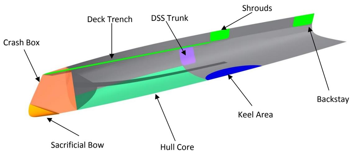
Figure 29: Area of Local Reinforcement
