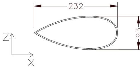
Figure 35: Spreader Mid Section (Dimensions in mm)
