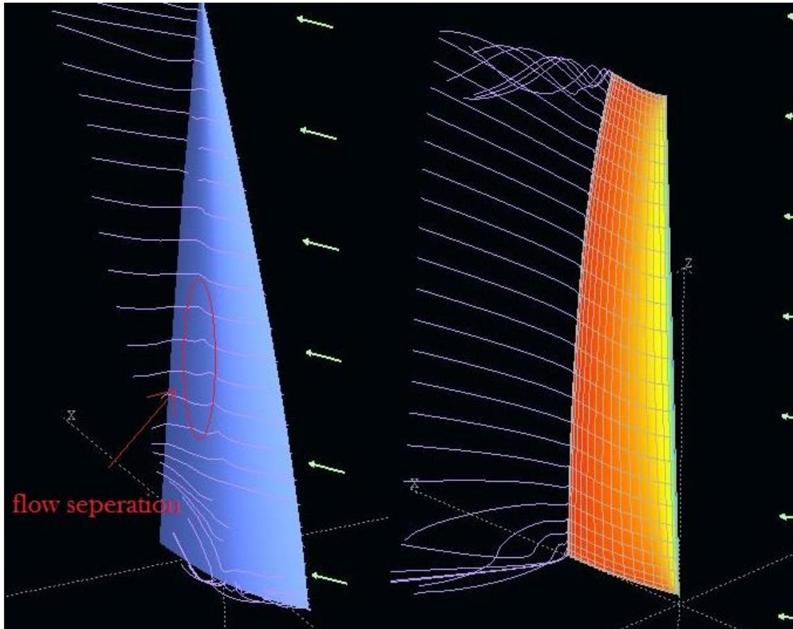
Figure 39: Streamlines Around the Mainsail and Jib
