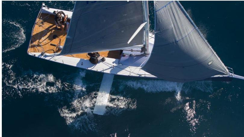
Figure 12: Existing DSS foil technology as seen on an Infiniti Yacht
