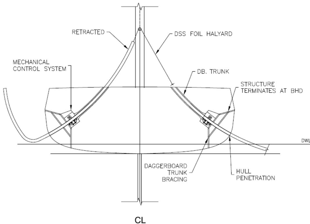
Figure 54:DSS Foil, Body Plan
