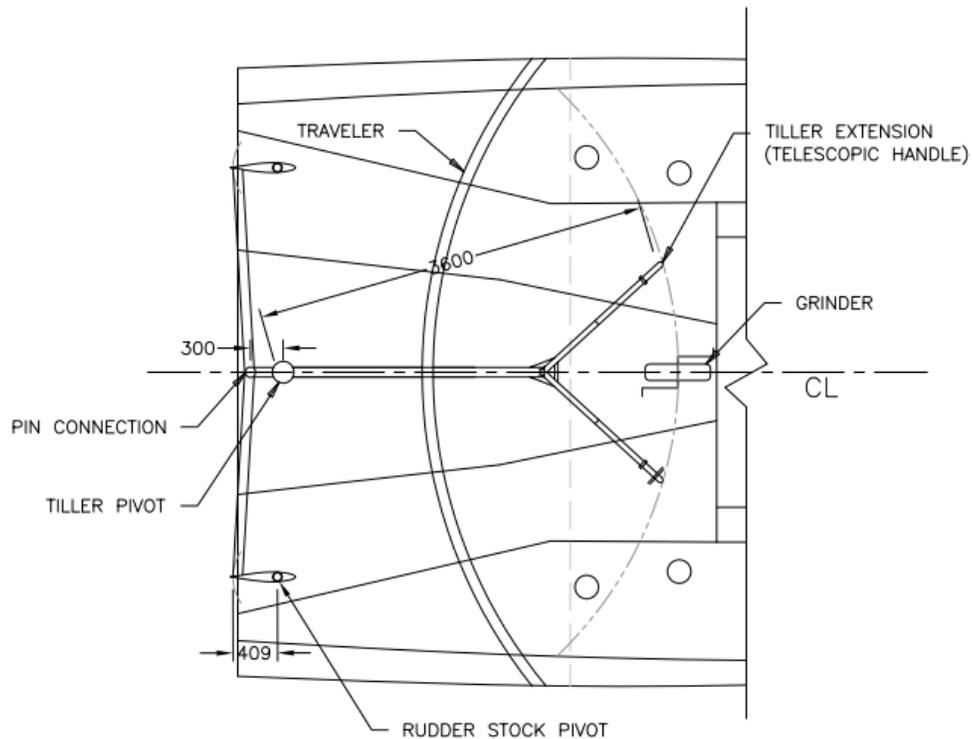
**Figure 32: Steering System (Dimensions in mm)**
