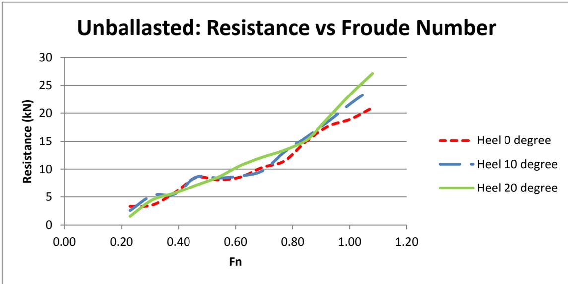
Figure 19: Resistance vs Froude Number in Unballasted condition
