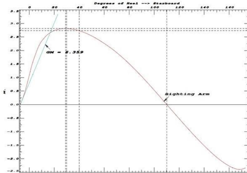
Figure 10: Righting Arm curve for 38 degrees cant
