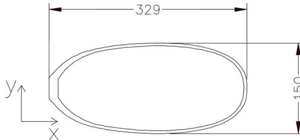
Figure 33: Mast Cross Section (Dimensions in mm)
