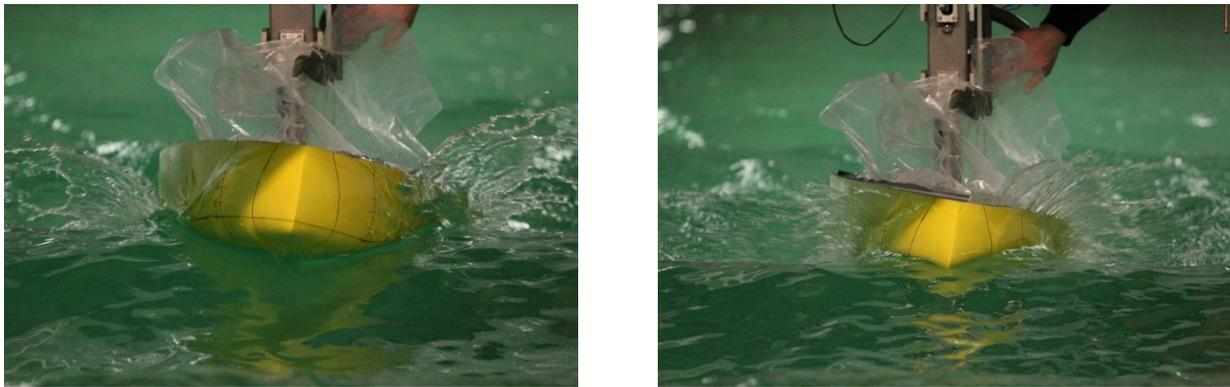
Figure 24: Ballasted condition with 10 degree heel and 0.8 Hz wave at 14 knots (left) and 18 knots (right). (Photo Credit to Ryan Williamson)
