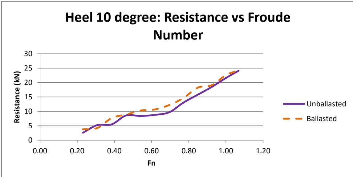
Figure 17: Resistance vs Froude Number at 10 degrees heel
