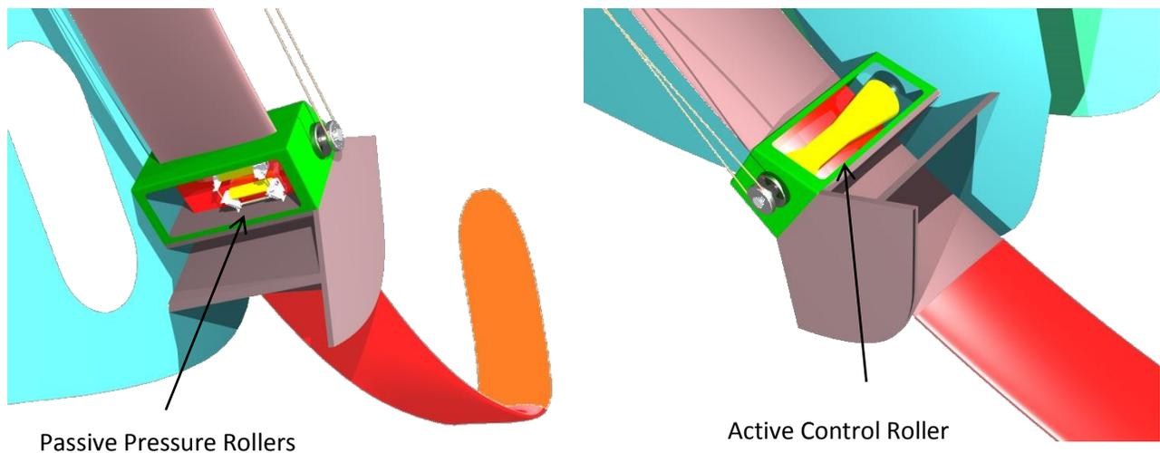
Figure 56: DSS Foil Lifting System (Top and Bottom Views)
