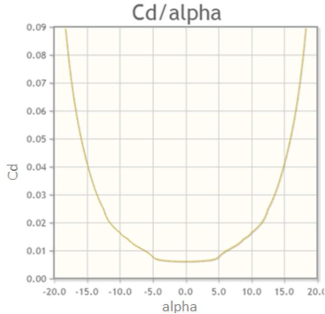
Figure 30: Selected foil section: NACA 63 A015 foil section with Reynolds number of  $1 \times 10^6$  (NACA 63-015A AIRFOIL, 2015)
