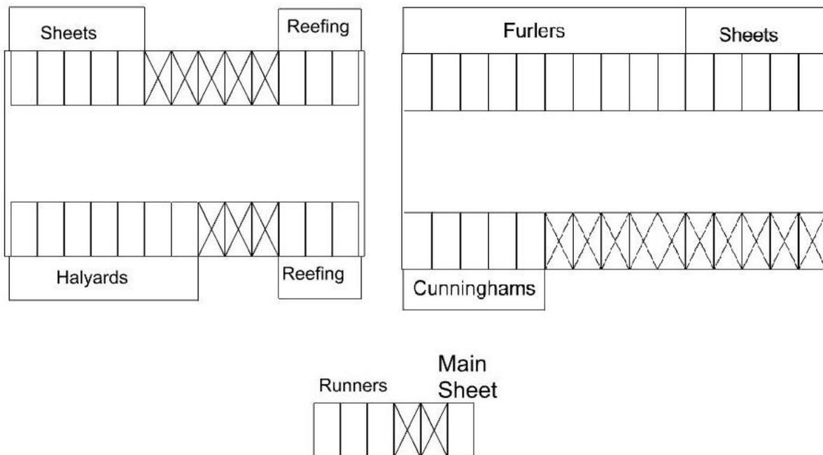
Figure 42: Arrangements of Cleats, top left is port, top right is starboard, bottom center is aft port and starboard, X implies spare cleats
