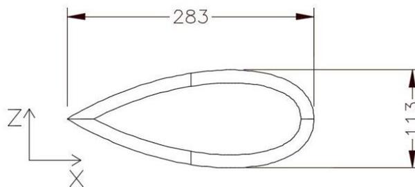
Figure 36: Spreader Mast Section (Dimensions in mm)
