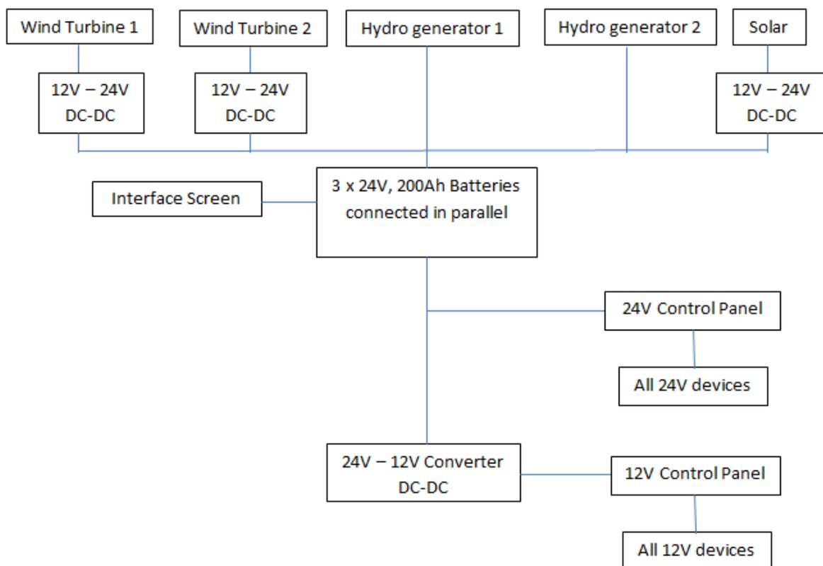
Figure 63: Electrical System Block Diagram
