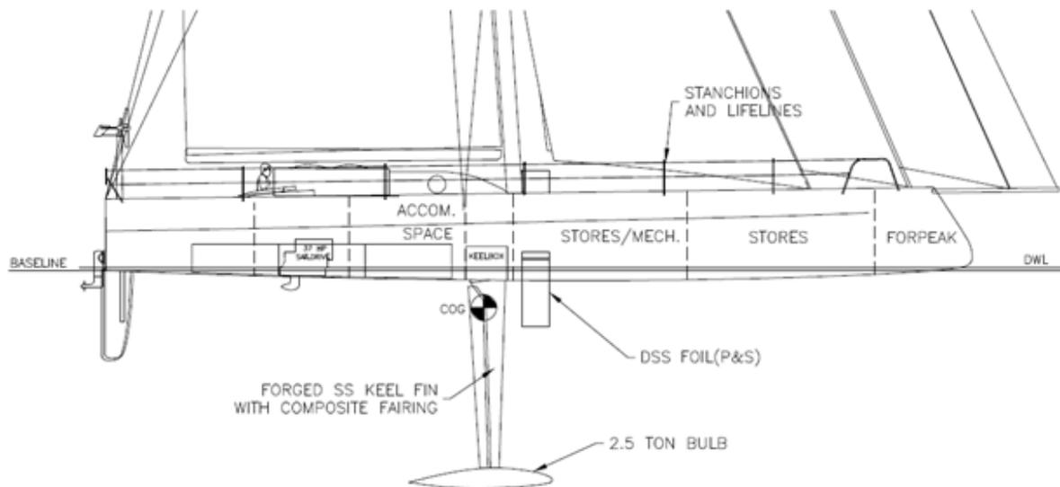
Figure 5: Profile view of The Type 600 Project
