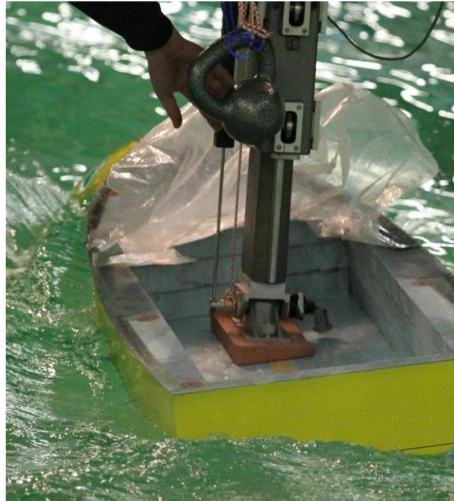
Figure 15: 10 Degree Heel Block Set Up
