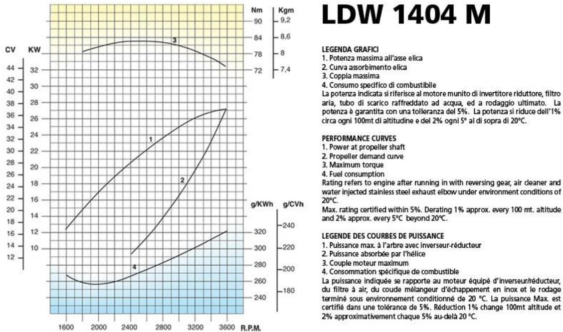
Figure 64: LDW 1404M 37 hp engine powering curves (ref: <http://www.lombardinimarine.com/download/curva1404m.jpg>)
