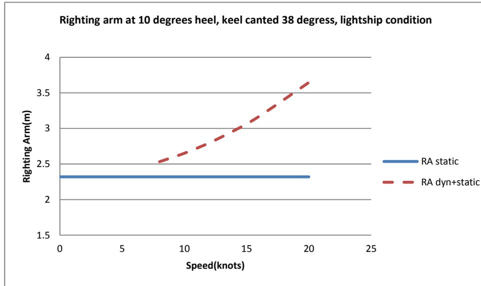
Figure 13: Static and Dynamic Righting Arm as speed increases
