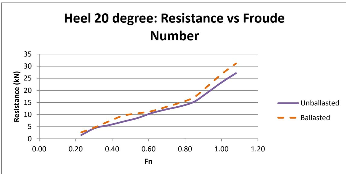
Figure 18: Resistance vs Froude Number at 20 degrees heel
