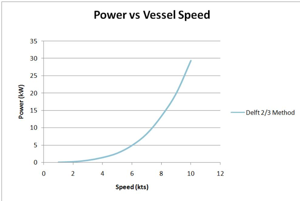
Figure 66: Power Required vs Ship Speed
