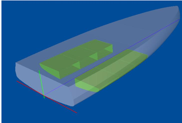
Figure 11: Ballast Tank Arrangement in Stability Model
